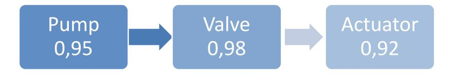
$$R(system) = R(pump) \cdot R(valve) \cdot R(actuator)$$
